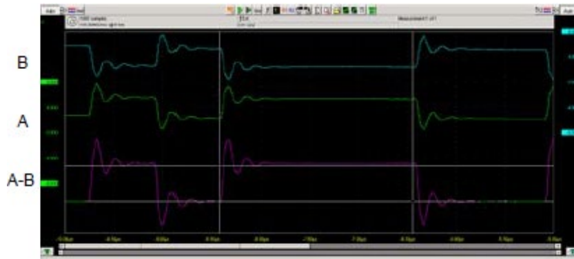
Fig. 9. Scope of signal with reflections
